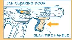
SLAM FIRE HANDLE must be pulled all the way back to open JAM CLEARING DOOR.
